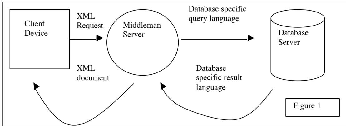
The above diagram (figure 1) shows the lifespan of a query, generated at the client device, processed by the Middleman server, and passed on to the database. The result of the query is passed back through the Middleman, additional processing is done, and the adapted result is then passed back to the client.
