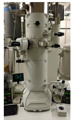
• In case of a dire emergency (eg sparks, fire), close the gun valve and leave the room immediately closing all doors behind you. When it is safe to do so call 911 and then the Campus Police. Finally, contact the facility staff. Do not attempt to shut down the instrument.
