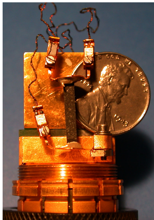
Fig. 1. Thermal conductivity sample (NWA 7309) attached with Ag epoxy and mounted on QD-PPMS TTO measurement puck. The Lincoln penny is added as a scale reference. (Color figure can be viewed at wileyonlinelibrary.com .)
