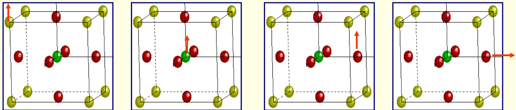
(Displacement pattern for cubic perovskite)
