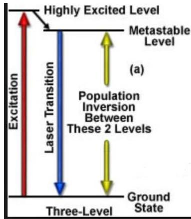
Figure 1. Three Level energy diagram - one of the many possible sets of energy level transitions that can result in laser action.
