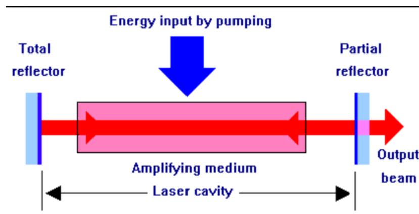
Figure 2. Diagram of Laser Optical Cavity
